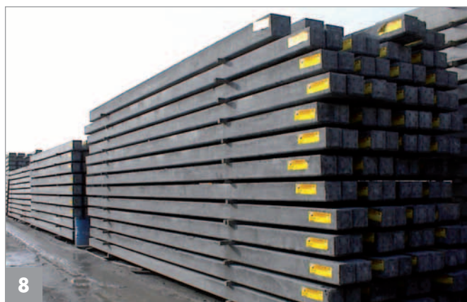
8 Foundation piles produced with fly ash concrete (source: Lodewikus Vorgespannen Beton/The Netherlands)
