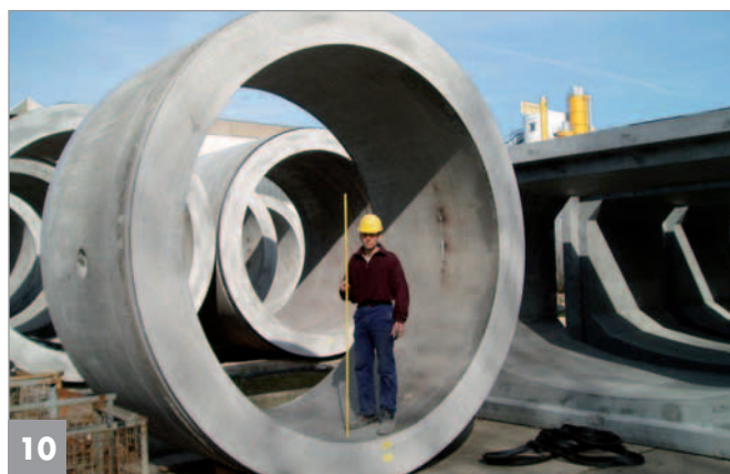
10 Jacking pipe made from acid resistant reinforced concrete (XA2) with fly ash and silica fume (source: BERDING Beton/Germany)
